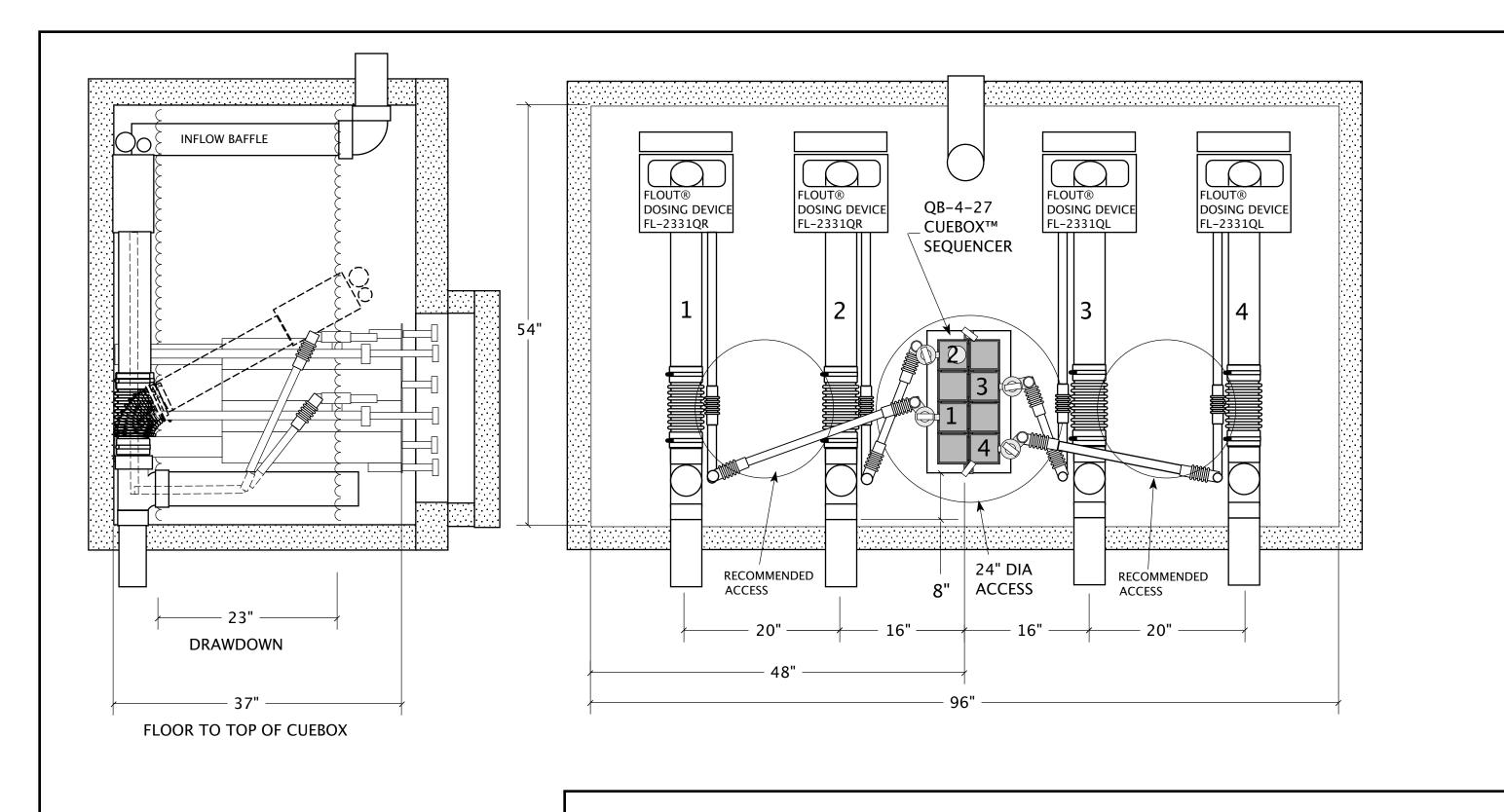
A PROPOSED DOSING CHAMBER WITH FOUR FLOUT® DOSING DEVICES EACH WITH ONE 3 INCH DIAMETER OUTLET. DOSING SEQUENCE CONTROLLED BY A CUEBOX™ SEQUENCER. 23 INCH DRAWDOWN.
